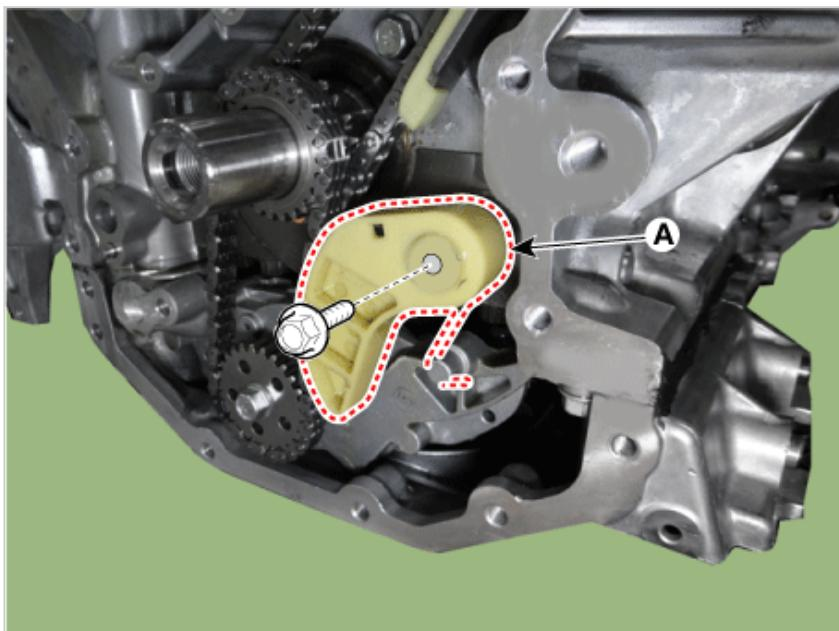
3. Remove the oil pump chain sprocket mounting bolt (A).
