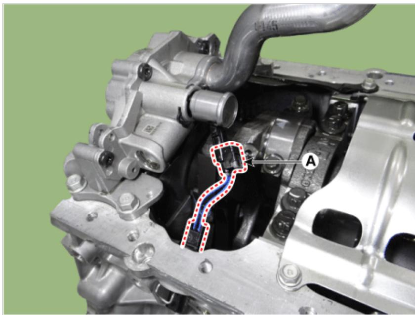
6. Remove the oil pump (A).
